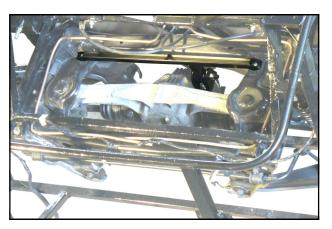
The crossbar is placed on top of the frame and bolted to the **U** bracket.
